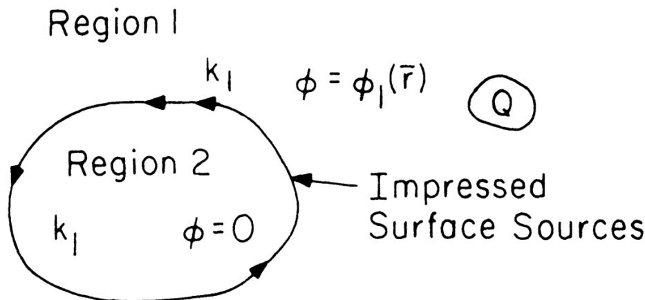
Figure 8.1.2 The illustration of the extinction theorem.
