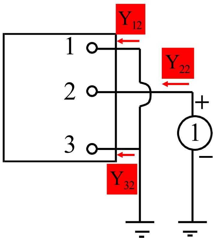
$$\begin{bmatrix} \dot{i}_1 \\ \dot{i}_2 \\ \dot{i}_3 \end{bmatrix} = \begin{bmatrix} Y_{11} & Y_{12} & Y_{13} \\ Y_{21} & Y_{22} & Y_{23} \\ Y_{31} & Y_{32} & Y_{33} \end{bmatrix} \begin{bmatrix} \dot{U}_1 \\ \dot{U}_2 \\ \dot{U}_3 \end{bmatrix}$$
