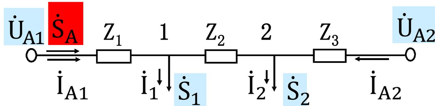
$$(U_{A1}^* - U_{A2}^*) \dot{U}_N = \dot{S}_{A1} (Z_1^* + Z_2^* + Z_3^*) - \dot{S}_1 (Z_1^* + Z_2^*) - \dot{S}_2 Z_3^*$$
