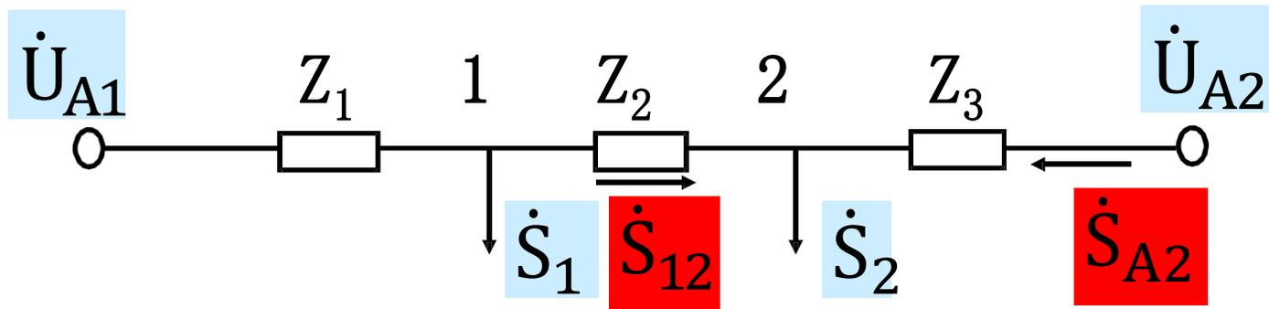
$$\dot{S}_{A2} = \frac{\dot{S}_1 Z_{I}^* + \dot{S}_2 Z_{II}^*}{Z_{\Sigma}^*} + \frac{U_N (U_{A2}^* - U_{A1}^*)}{Z_{\Sigma}^*}$$
