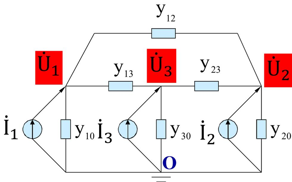
$$\begin{bmatrix} \dot{I}_1 \\ \dot{I}_2 \\ \dot{I}_3 \end{bmatrix} = \begin{bmatrix} Y_{11} & Y_{12} & Y_{13} \\ Y_{21} & Y_{22} & Y_{23} \\ Y_{31} & Y_{32} & Y_{33} \end{bmatrix} \begin{bmatrix} \dot{U}_1 \\ \dot{U}_2 \\ \dot{U}_3 \end{bmatrix}$$
