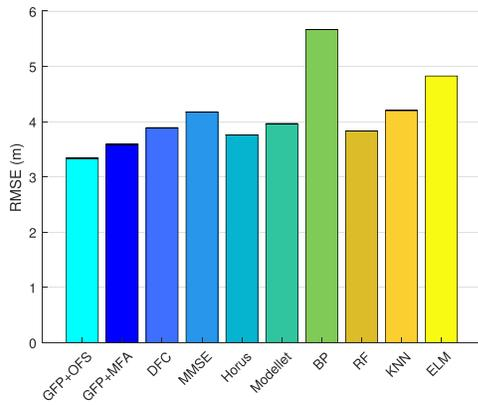
Fig. 10. Histogram of average RMSEs of different localization algorithms.
