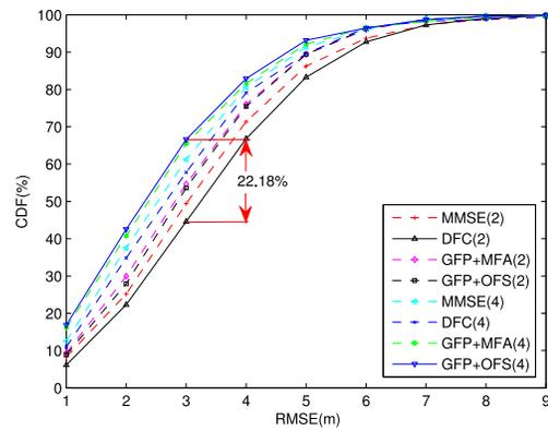
Fig. 6. CDFs versus RMSEs with different number of fingerprint functions.
