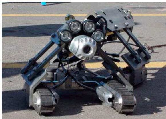
**Figure 5.** Closed-circuit television camera (CCTV) pipeline inspection from [144]. (Reprinted with permission from ref. [144]. Copyright 2021 Elsevier).
