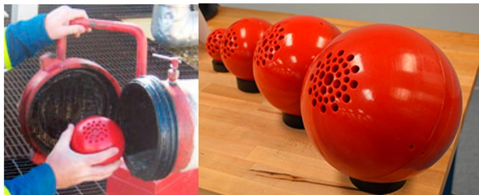
(a) Smart ball for pipeline inspection
